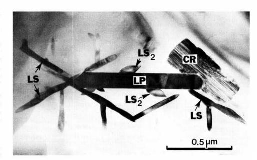
ELECTRON MICROGRAPH confirms long-suspected epitaxial growth on precipitates with an oxide nucleating agent; here, cristobalite (CR), lithium metasilicate (LS), and lithium disilicate (LS $_2$ ) grow on the exposed faces of a lithium phosphate (LP) crystal in Sandia-developed S-glass, a glass-ceramic containing  $P_2O_5$  nucleating agent.
